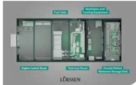
Top view of the rendered CAD model incl. the room designation.
