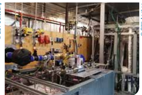
Test bench with MultiSchIBZ solid oxide (SOFC) fuel cell system in the OWI laboratory
